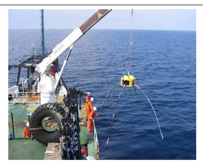
Receivers detect and record electric and magnetic fields at the seafloor. Deployed autonomously and recovered using acoustic release system
