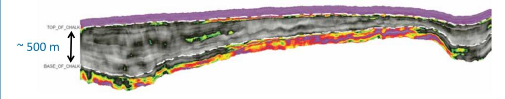
• Seismic inversion can be used to find porous zones, but determining the fluid content is difficult.
