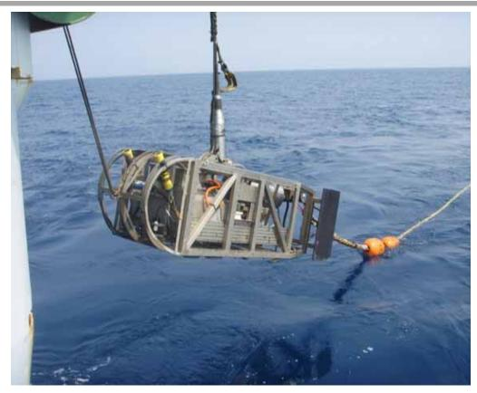
High powered dipole source with a moment in excess of 300,000 Am in the fundamental.
